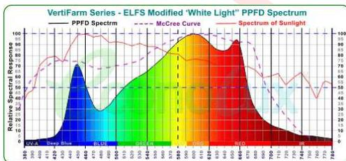
The VertiFarm-40 and VertiFarm-60 lights are available with a standard ELFS spectrum which is based on the popular modified 'White Light', good enough full spectrum, with output throughout the PAR range from 400nm to 750nm. This spectrum has a good balance between the ideal spectrum (McCree curve) and cost, with a 70% match to the McCree curve.
